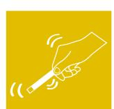
2. Shake the strip to remove any excess solution. In some tests this step may not be necessary.
